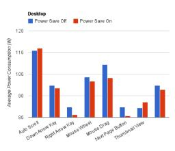
Figure 2: Average Power Consumption values for the Desktop Condition.
