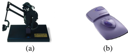
Figure 1. (a) SensAble PHANToM, (b) WingMan force feedback mouse.
