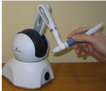
Figure 3: A picture of a SensAble Technologies’ PHANTOM Omni haptic device as used in the Graph Builder application. The user interacts with the ‘pen’ which also contains two buttons for interaction.
