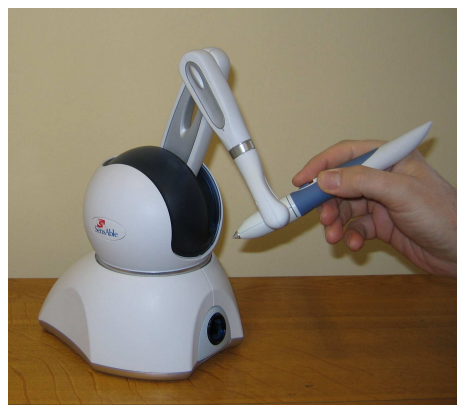
Figure 1: A picture of a SensAble Technologies’ PHANTOM Omni Haptic Device. The use of motors and optical sensors allows the user to “feel” virtual objects.
