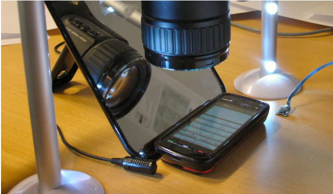
Figure 10. Close-up of the mirror arrangement. The microphone (front) and the accelerometer (back) are not attached to the phone in this figure.
