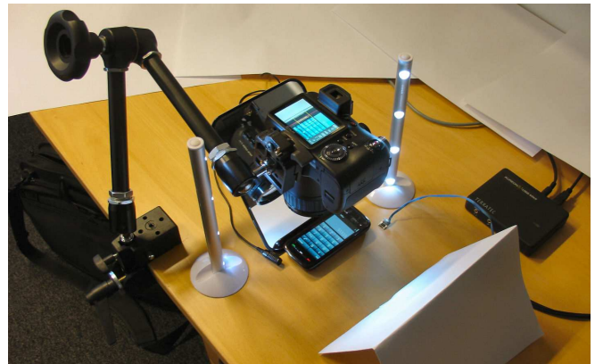
Figure 1. Overall setup of the multimodal latency measurement tool.
