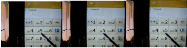
Figure 7. A picture sequence showing the stylus approaching and finally touching the touchscreen surface of a mobile phone. The mirror can be seen on the left and gives a clear view of when the stylus hits the screen. The picture is of the Samsung Omnia i900 dialler user interface.
