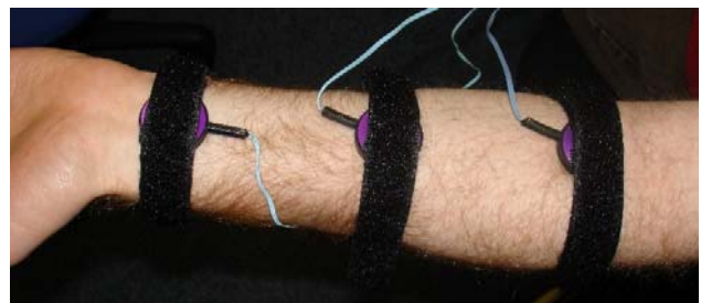
Figure 6: The location of the Tactors on the participant's forearm.
