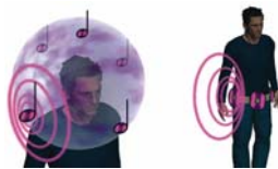
Figure 1. 'turn right' cue indicated by audio panned to the right (Earcon) and activation of factor on right hand side of waist (Tacton).
