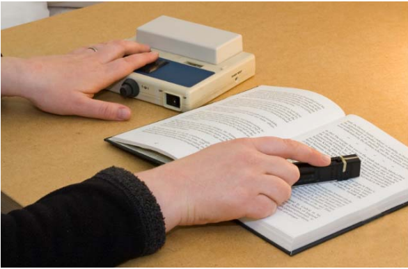
Figure 2: Using the Optacon device to read text. A handheld camera detects light and dark areas of the page and converts to a vibrotactile pictorial representation, presented to a finger on a vibrating array.
