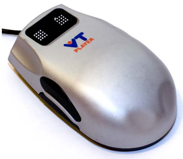
Figure 3: The VTPlayer tactile mouse. A tactile display with two 4 by 4 arrays of pins.
