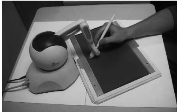
Fig. 10. New pen attachment to replace the large PHANTOM Omni pen shaft.
