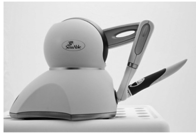
Fig. 3. SensAble Technologies PHANTOM Omni force-feedback haptic device ( www.SensAble.com ).
