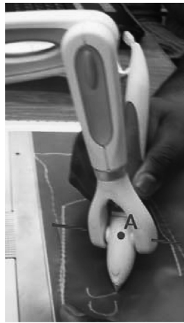
Fig. 11. Point A (the gimbal) is the standard point of control when using the PHANTOM, rather than the tip of the pen on the writing surface.
