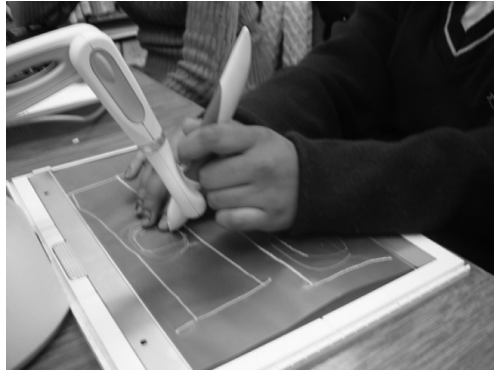
Fig. 9. A totally blind participant using the PHANTOM—Note the nonwriting hand used to feel the tactile line that has been drawn on the drawing board.
