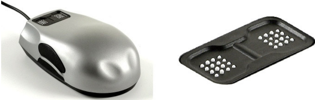
Figure 6. The VTPlayer mouse developed by VirTouch. The right hand image shows the two arrays of blunt pins.
