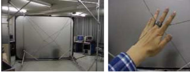
Figure 13. The scalable SPIDAR force feedback device is shown on the left. The right picture shows a user interacting with the SPIDAR.
