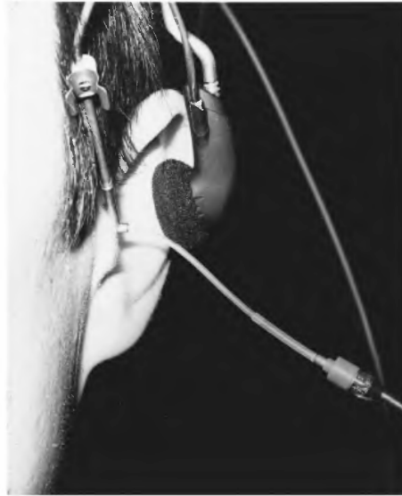
Figure 8. The acoustically open transducer used by Langendijk and Bronkhorst. The transducer is positioned at a distance to the ear to allow for a microphone to be placed in the ear.
