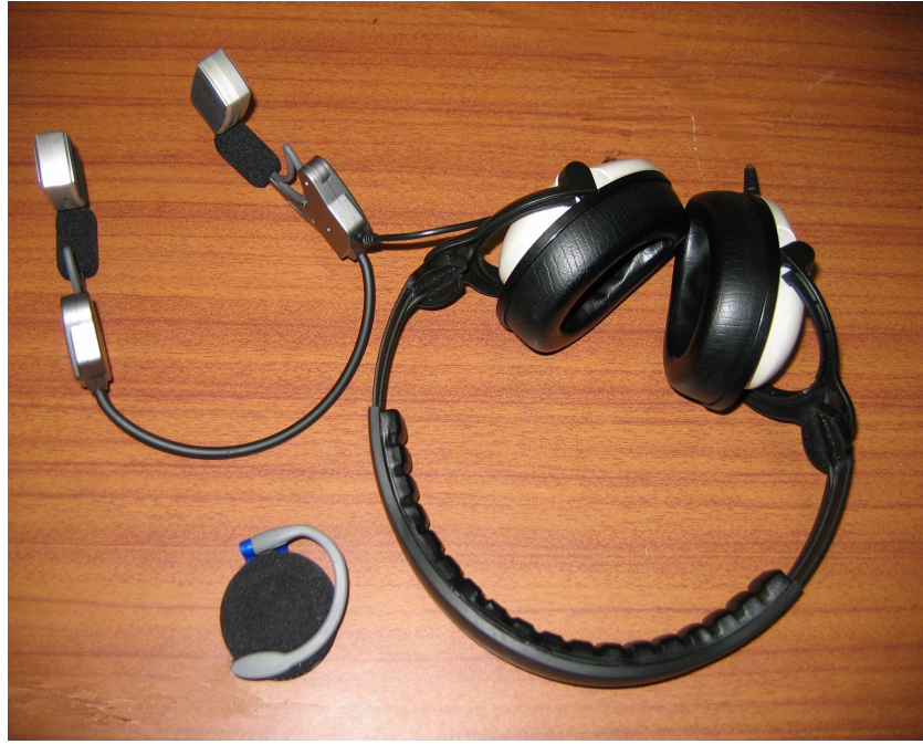
Figure 32. The different headphone types used in the experiment, bottom left is the single earpiece (Panasonic RP-HS50), top left are the bone conduction headphones (Vonia EZ – 3200P) and to the right are the Sennheiser HD 200 headphones.
