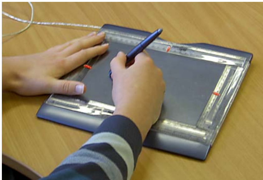
Figure 6. Graphics tablet augmented with a tangible frame delimiting the working area. Red tangible dots can be seen indicating the midpoint of every side of the rectangle. In the image, a user feels the tangible frame with the left hand while moving the electronic pen over the working area with the right hand.
