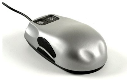
Figure 3. Close up of a pin array from VirTouch's VTPlayer mouse [159].
