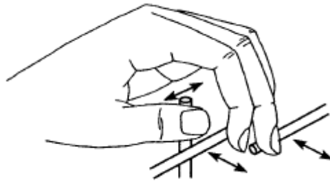
Figure 3-1: Schematic drawing showing the placement of the fingers of the Tactuator device, and the available motions, from [106].
