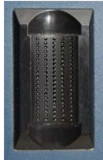
Figure 3-2: Using the Optacon device to read text. The image on the right shows a close-up of the pin array.
