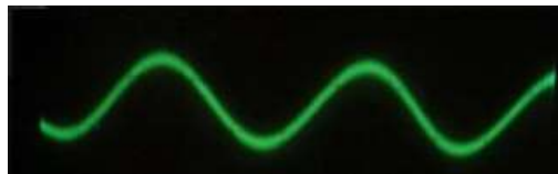
Figure 5-1: Output of TACTAID VBW32 when a sine wave was input.
