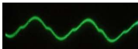
Figure 5-2: Output of TACTAID VBW32 when a square wave was input.
