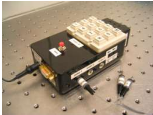
Figure 7-3: "Tacton Box" with numeric keypad: hardware for creating and presenting Tactons via a standard phone vibration motor.
