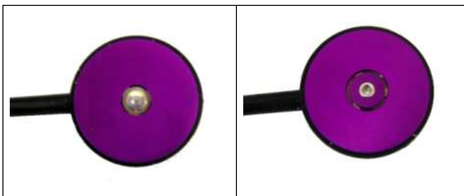
Figure 5-7: The C2 Tactor in the “indented” orientation (left) and in the “raised” orientation (right)
