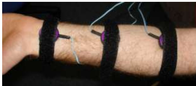
Figure 8-3: The location of the Tactors on the participant's forearm.
