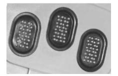
Figure 1. A tactile pin array for fingertip display, consisting of three 4 x 8 arrays of pins.
