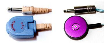
Figure 2: Left – a TACTAID VBW32 transducer, right an EAI C2 Tactor.
