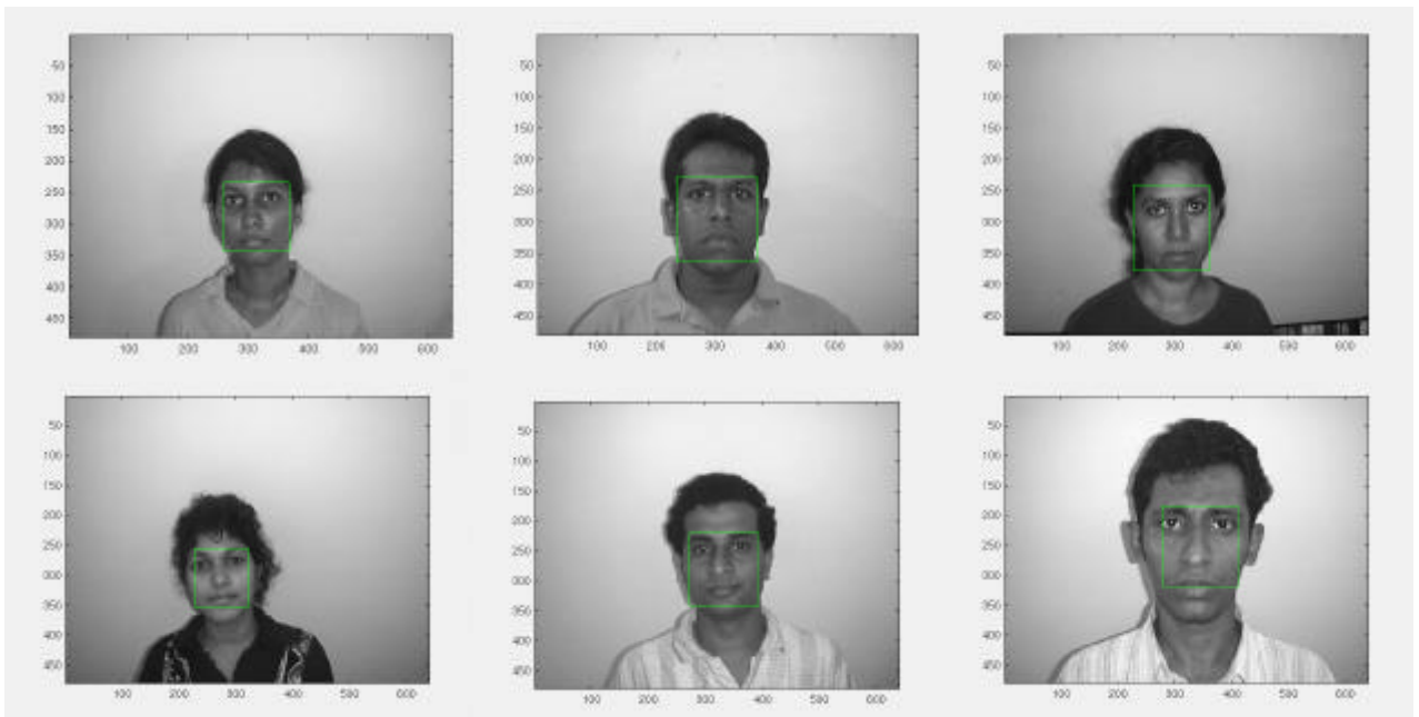
Figure 6.2 The 6 good face segments from 27 condition A images. All other face detections resulted in excellent face segments. Many of the above were not segmented perfectly because the subject's head was slightly at an angle or like in the lower right figure, the subject was not perfectly symmetrical.
