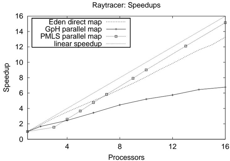
Figure 32. Speedups for `raytracer` on the Beowulf
