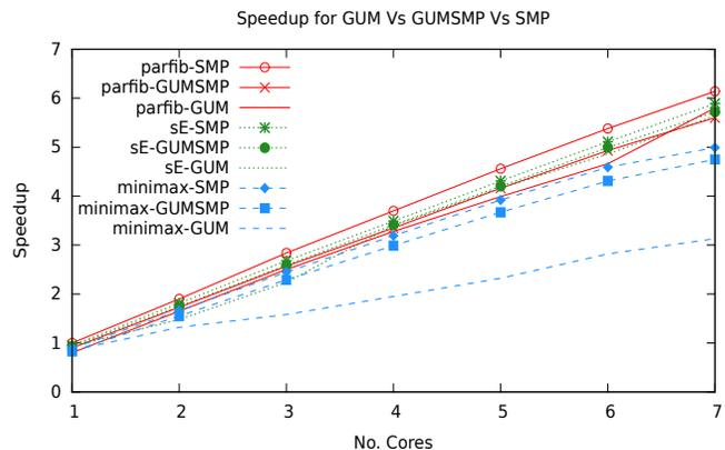
Figure 7: Speedup of all programs using GHC-GUM, GUMSMP, and GHC-SMP on a *single multi-core*
