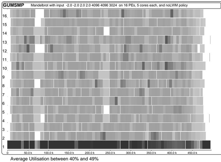
Figure 9: mandelbrot load distribution without low-watermark on GUMSMP
