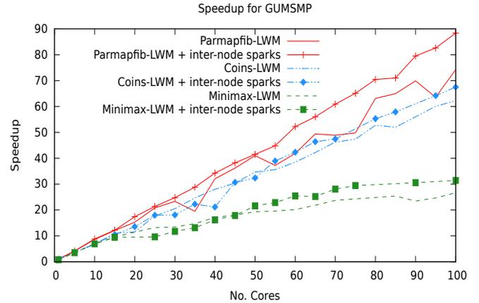
Figure 12: Speedups of GUMSMP using an *asymmetric load distribution policy*, enabling inter-node sparks
