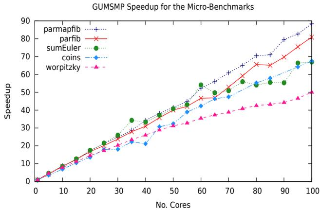
Figure 5: Speedup of *micro-benchmarks* using GUMSMP
