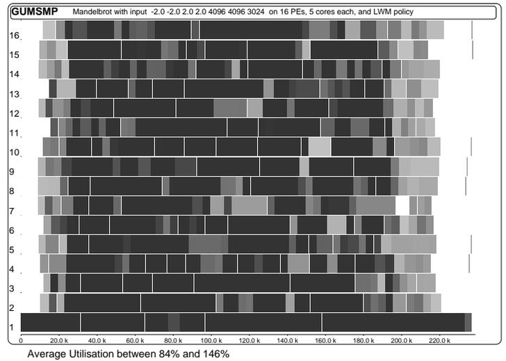
Figure 10: mandelbrot load distribution with low-watermark on GUMSMP
