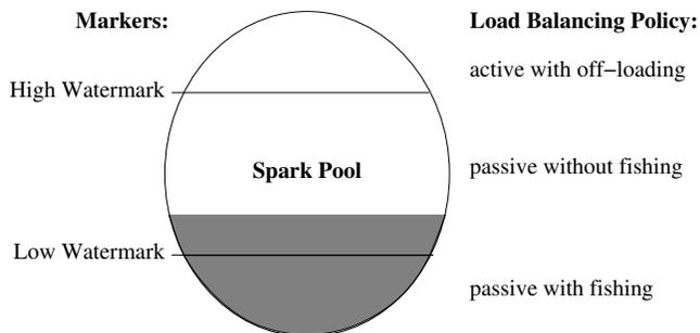
Figure 4: Low- and High-watermark mechanisms for spark distribution.
