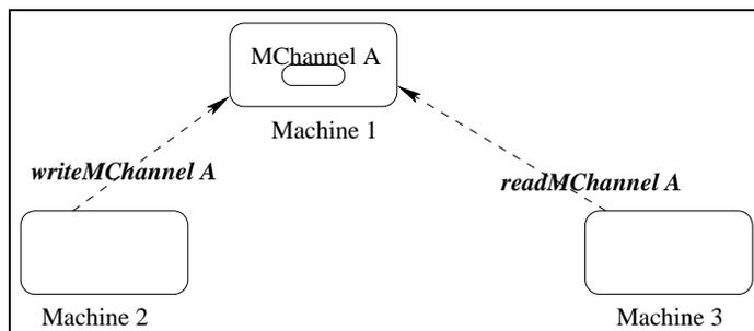
**FIGURE 1.7. Machines 2 and 3 cannot communicate if Machine 1 crashes**
