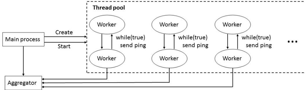
Figure 2. Design of the Concurrent Process Throughput Benchmark
