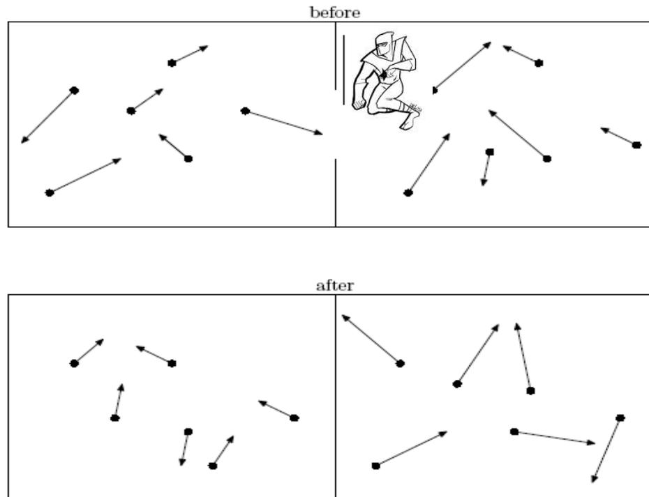
**Gas initially in equilibrium. Daemon opens door only for fast molecules to go from A to B, or slow ones from B to A. ! Slow molecules in A, fast in B. B hotter than A, and can be used for power.**
