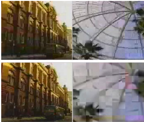
Figure 5: The upper pair of images show successive frames with the rate control algorithm described in the paper. The lower pair show the same frames at the same average bit rate of 2400 bits per frame but with a constant number of bits per frame.
