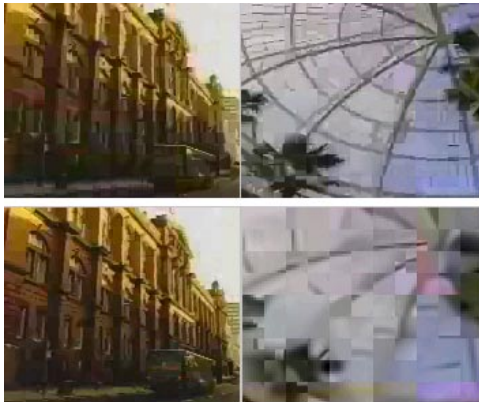
Figure 5: The upper pair of images show successive frames with the rate control algorithm described in the paper. The lower pair show the same frames at the same average bit rate of 2400 bits per frame but with a constant number of bits per frame.
