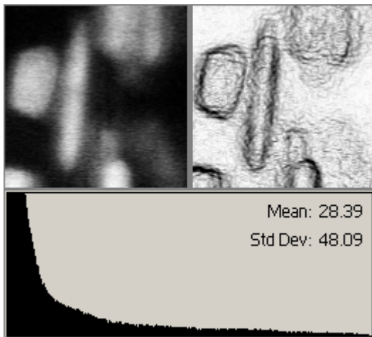
(b-1) An 128 x 128 area clipped from the 41st frame from original image data set as shown top left corner. The result of edge-detection filter is shown on its right side. The histogram of the entire frame is shown on the lower part.
