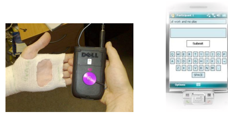
Figure 1: Experiment set-up with PDA, C2 Tactor, bandage securing the SHAKE to hand and text entry GUI screenshot.
