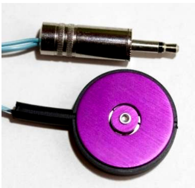
Figure 4: The C2 Tactor from Engineering Acoustics ( www.eaiinfo.com ).
