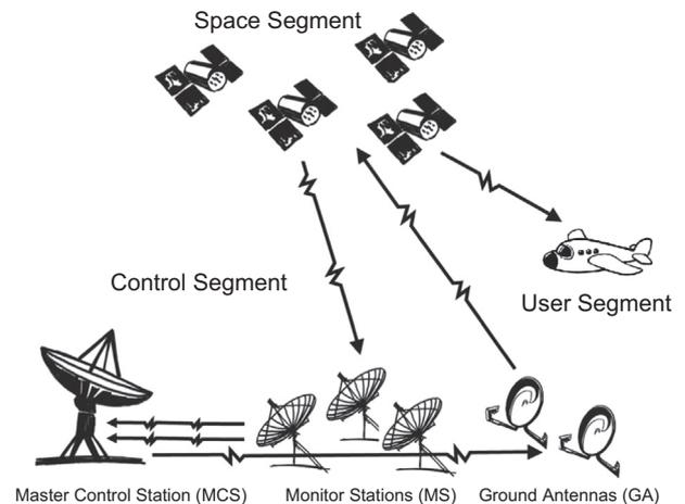
Fig. 2. Three segments of a GNSS system.
