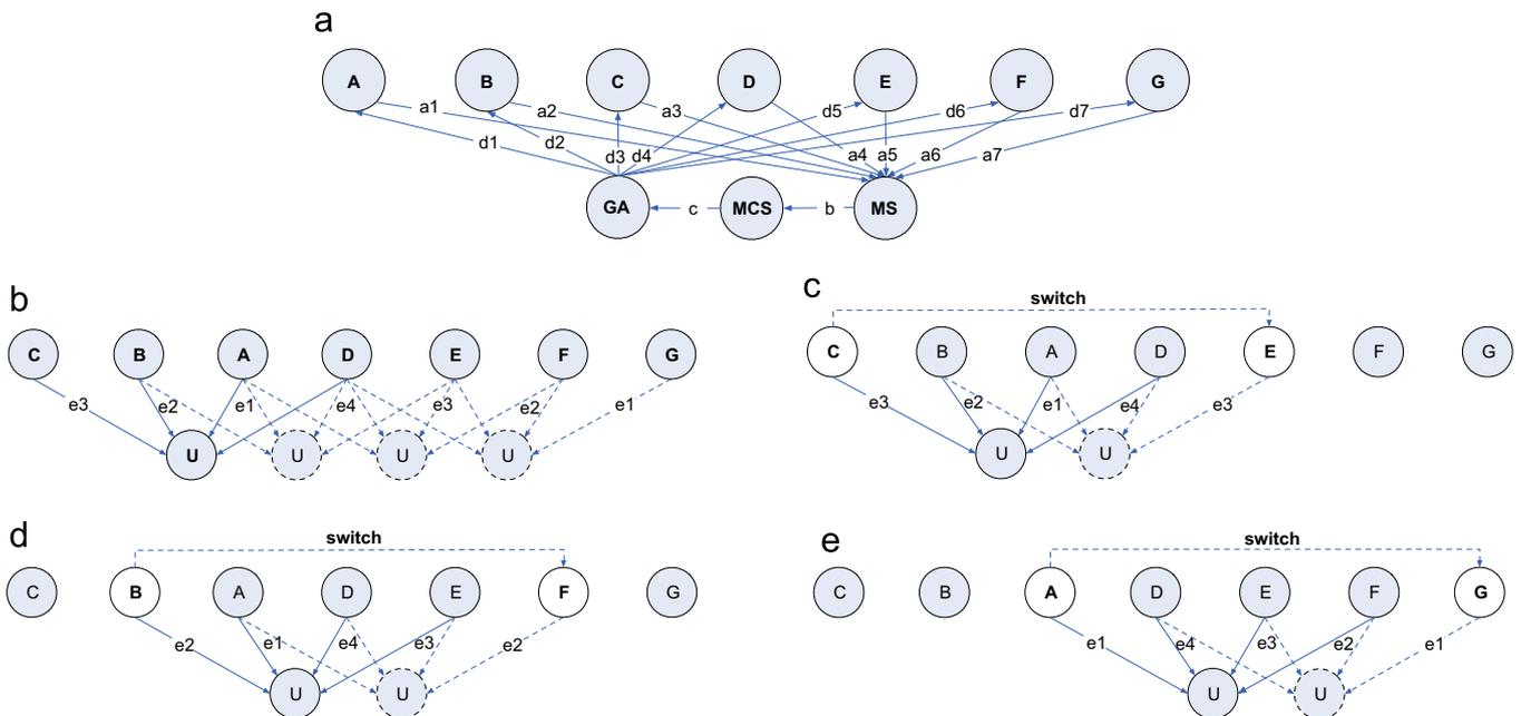
Fig. 10. Reference Model of GNSS Segments. (a) Reference model of control and space segments. (b) Reference model of user and space segments. (c) Switch satellite C with E. (d) Switch satellite B with F. (e) Switch satellite A with G.
