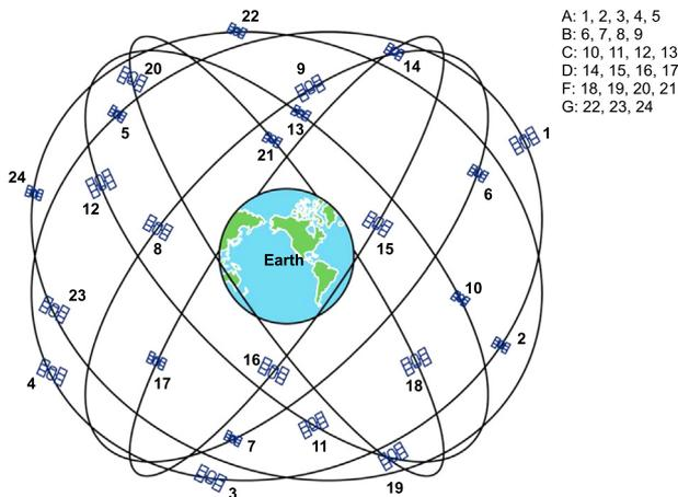
Fig. 3. A GNSS consisting of a constellation of 24 satellites.
