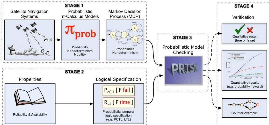
Fig. 5. Stages in probabilistic verification.
