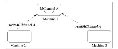
FIGURE 1.7. Machines 2 and 3 cannot communicate if Machine 1 crashes
