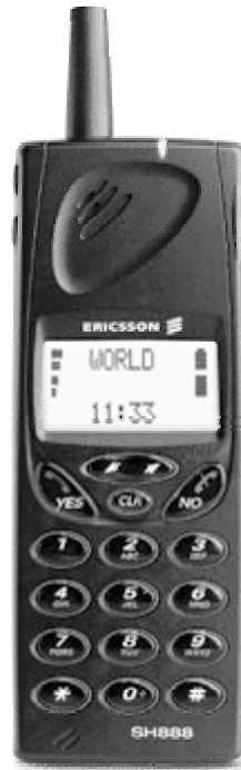
Figure 2. The keypad and the various function keys (YES, NO, CLR and arrow keys (down/up) encountered on an Ericsson 888 cellular terminal.
