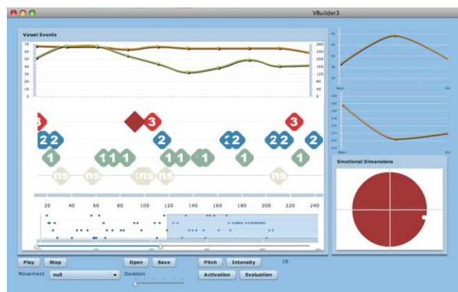
Fig. 2. Prototype of the acoustic analysis viewer. Pitch and intensity curves are displayed at the top, with all vowels present displayed relative to their prominence in the middle chart. The pitch and intensity curves for the current vowel are displayed in the right, as are the emotional dimensions for the current asset.
