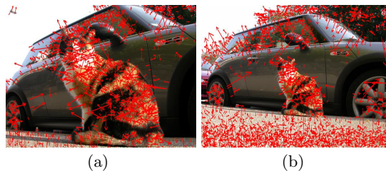
Fig. 2. The 1481 SIFT keypoints extracted from the query image (a) and a very similar image of same size with 2536 keypoints (b) to which we will later on compare it.
