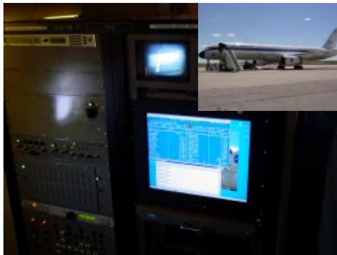
Figure 2 – Data Acquisition System (DAS) onboard the NASA B757 ARIES aircraft (inset).
