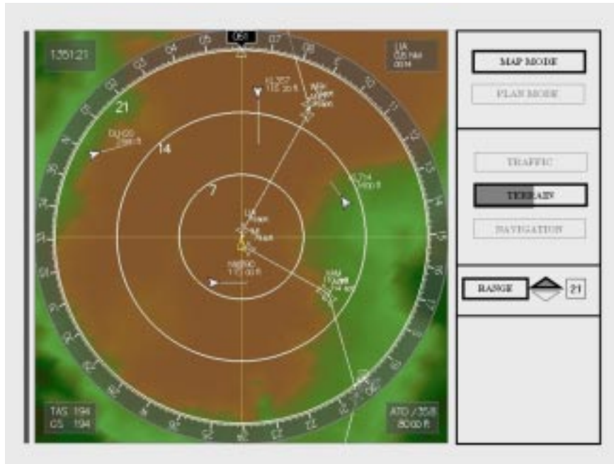
Figure 2: An impression of the intelligent Navigation Display. The adaptation level shown is the interactive level that lies in between the proactive and reactive levels. It shows the operator what changes to the current display setting are required to get a good view on the conflict (in this case a terrain conflict).
