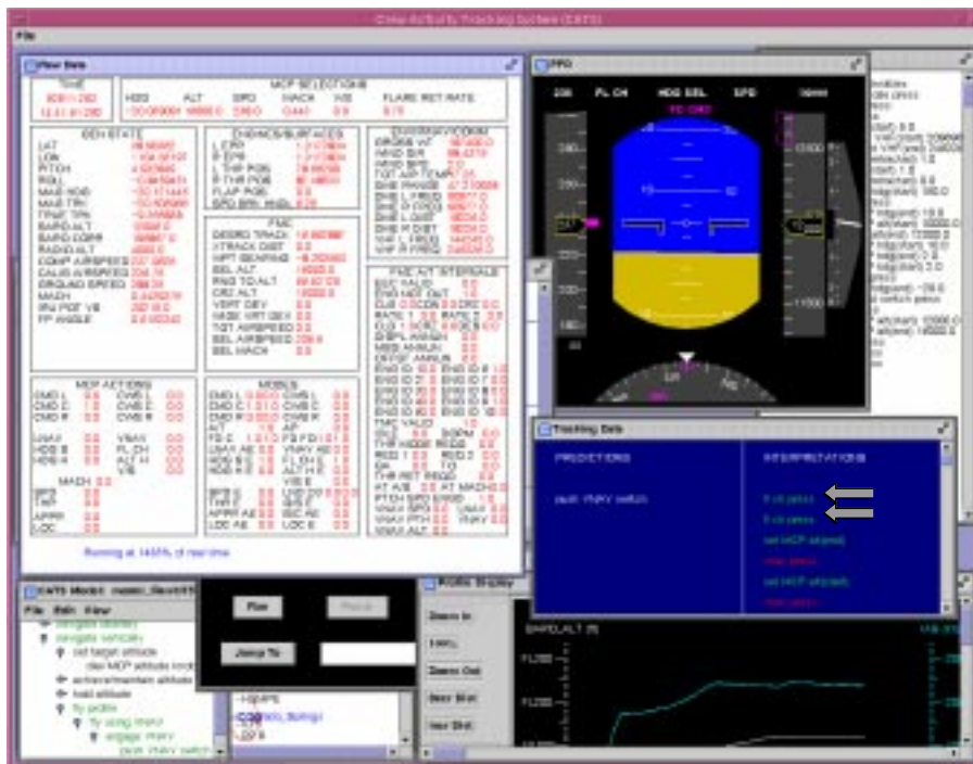
Figure 11 - Scenario Frame 7: CATS detects a second ‘insurance’ FL CH switch press, and interprets it as acceptable as it did the first FL CH switch press.
