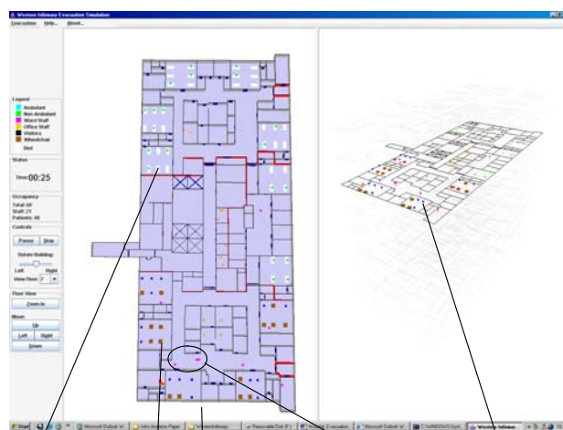
White rectangles show beds, brown squares are wheelchairs. Overhead plan of selected floor showing fire walls in red. Purple squares show ward staff coordinating evacuation. 3D Floor plan with current floor giving aerial view of evacuation
