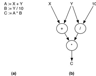
**Figure 3: A simple program (a) and its dataflow equivalent (b)**
