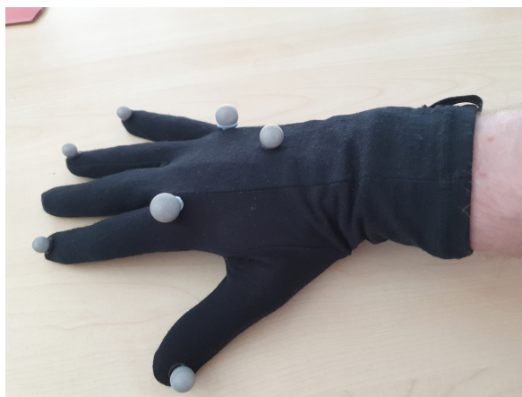
Figure 5.10: The 7 passive IR markers used to track hand motions.
