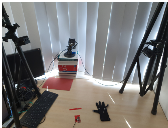
Figure 5.9: The OptiTrack recording setup showing the 3 cameras positioned around the workspace and the Soli board on the desk.
