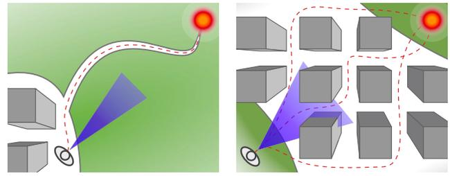
**Figure 1: Dynamic feedback is directly related to path options. When fewer routes are available (left) the feedback area (shown in blue) is small, expanding when there is more choice (right). The centre of the feedback area aims directly at the goal.**
