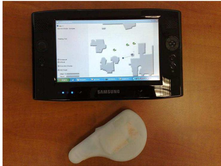
**Fig. 5.** A Samsung Q1 UMPC with a Bluetooth connection the WayStane inertial sensing device
