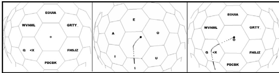
**Fig. 1.** The hexagonal layout. Each letter is assigned to a group, within which it is associated with a particular edge. In this example, producing “o” requires an upwards then up-right movement.
