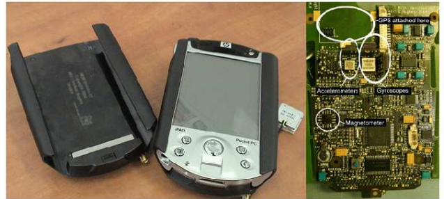
Figure 1: The MESH expansion pack, with an iPaq 5550 PocketPC. This provides accelerometer, gyroscope and magnetometer readings, as well as vibrotactile display.
