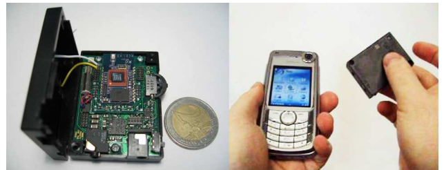
Figure 2: The wireless SHAKE sensor, shown with a 2 Euro piece and a Nokia 6660 for size comparison. This Bluetooth device comprises a complete inertial sensing platform with onboard vibrotactile feedback.
