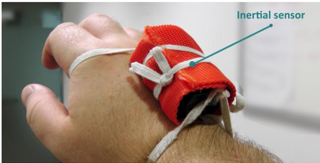
Figure 4: The SK7 inertial sensor, as mounted on the hand. The elastic mounting minimises slippage.
